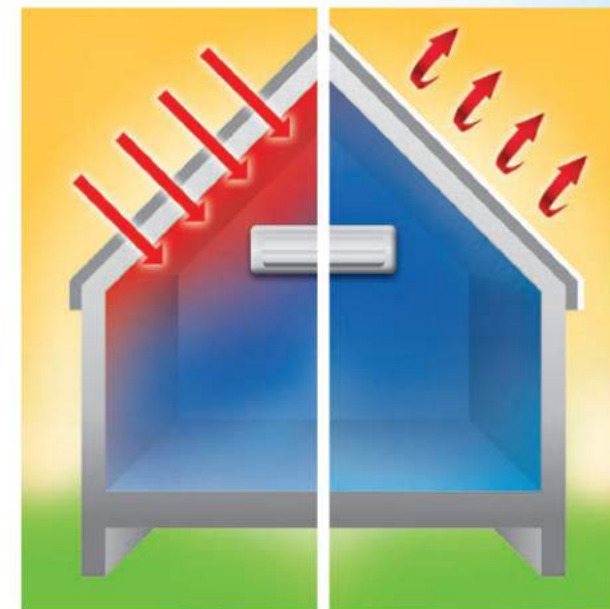
Transmission and reflection of heat waves without coating and with thermoreflexive coating KOFATERM ROOF
